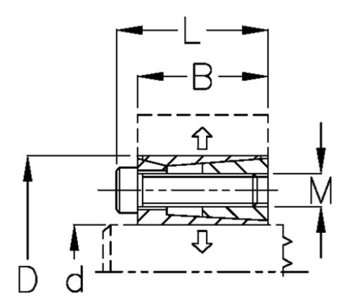
$\begin{array}{lll} \text{B mm} & = 28 \\ \text{d mm} & = 42 \\ \text{D mm} & = 70 \\ \text{Fit tolerance} & = \text{Aksel h8, Nav H8} \\ \text{F kN torque} & = 90 \\ \text{L mm} & = 36 \\ \text{M mm} & = \text{M8} \\ \text{P N/mm2 surface pressure on shaft/hub} = 135 \\ \end{array}$
